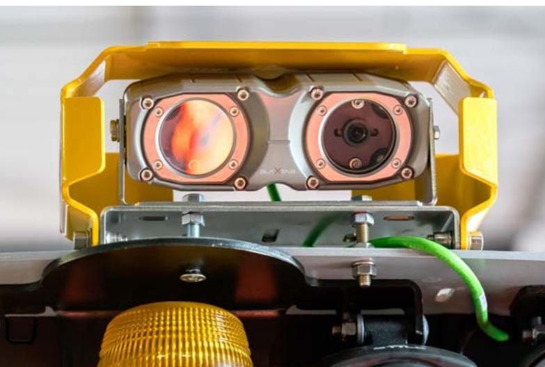
The Blaxtair reversing safety system from Arcure comprises a 3D sensor head, a calculator unit and a screen in the forklift driver's cab.
