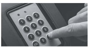
Another alternative is an individual five- or eight-digit PIN which the driver types in on a built-in keypad to conveniently activate the respective truck. All the driver has to do to log out is press the 'Escape' button.
