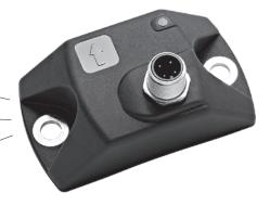
The 'shock detection' function helps to reduce unusual impact and to minimise the costs incurred as a result of impact damage. It consists of a sensor that measures vibrations in the truck. Should the vibrations exceed a certain level, the impact will be registered as unusual and the fleet manager is informed, who can then train the driver to handle the truck correctly.
