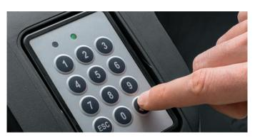
Another alternative is an individual five- or eight-digit PIN which the driver types in on a built-in keypad to conveniently activate the respective truck. All the driver has to do to log out is press the 'Escape' button.
