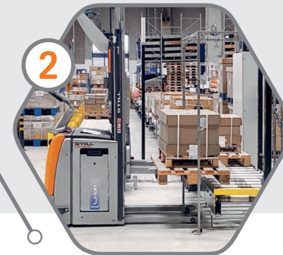
EXV iGo up to 3,744 mm up to 1.6 t up to 2.0 m/s
