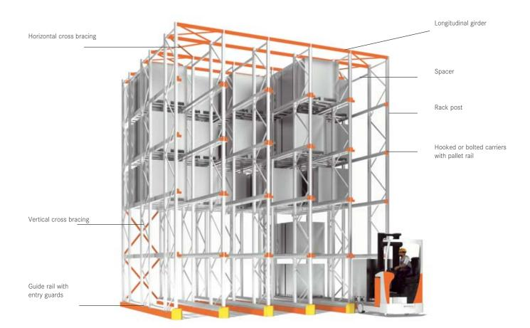
Drive-in racks from STILL are designed as drive-in or drive-through racks. Drive-in racks are loaded and unloaded from one side only. Drive-through racks can be accessed from both sides.
