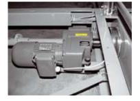
All electric drives are directly connected to the carriage drive shaft. The drive shaft is attached to the driving wheels by a flange coupling.
