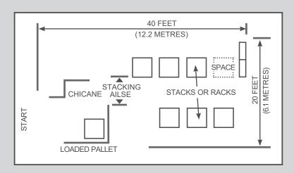
Plan of area required to conduct training on your premises. Area to be clear of obstacles in order that this test course can be used to the best effect. Larger area required for bigger trucks.
