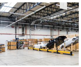
Trucks are constantly placing new containers in the allocated spaces. A few minutes later, one of the automated reach trucks arrives and takes the container to the rack.
