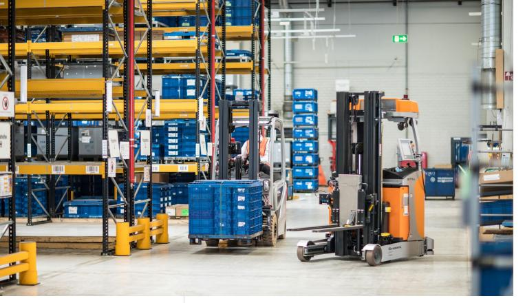
The automated FM-X trucks keep out of the way of the manually driven vehicles, with safety features such as sensors and acoustic signals preventing any collisions.
