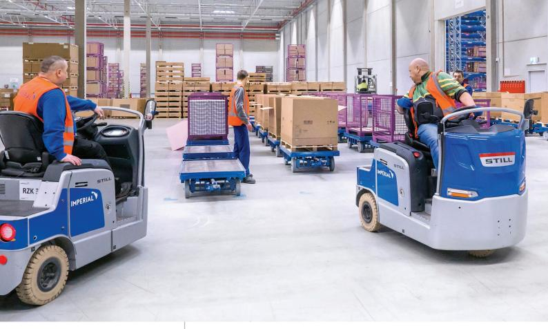
Cage pallets to re-pack goods for overseas shipments are moved with the electric LTX 70 tractors. They are outstandingly manoeuvrable and tow up to 8 tons.
