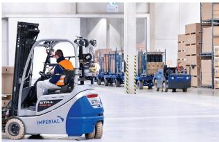
The powerful and robust R 07 tractors from STILL tow loads of up to 25 tons distributed on three trailers. Changing the battery over the side for fresh energy only takes a few moments.
