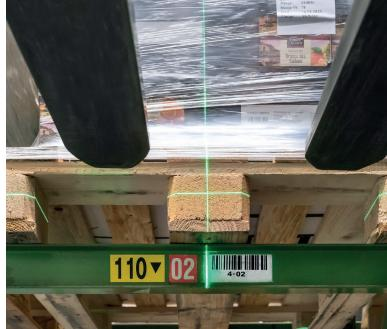
The visibility-optimised overhead guard increases safety and gives the driver optimum all-round visibility thanks to the slanted strut arrangement and the additional panoramic mirror.
