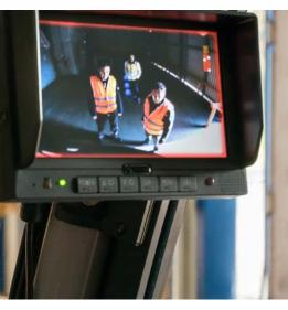
↑ Typical accident situation: A person enters the risk zone outside of the driver's field of vision. If there is a risk of collision with a person, an alarm is triggered immediately and the driving speed is reduced to creep speed.
