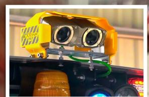
Camera system for forklift trucks: Safety system prevents accidents between people and forklift trucks when reversing.
