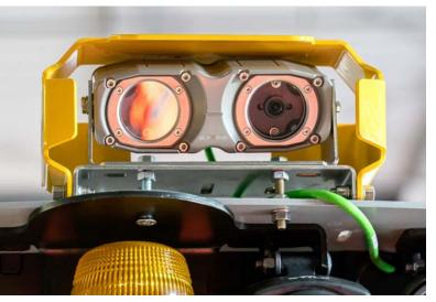
The Blaxtair reversing safety system from Arcure comprises a 3D sensor head, a calculator unit and a screen in the forklift driver's cab.
