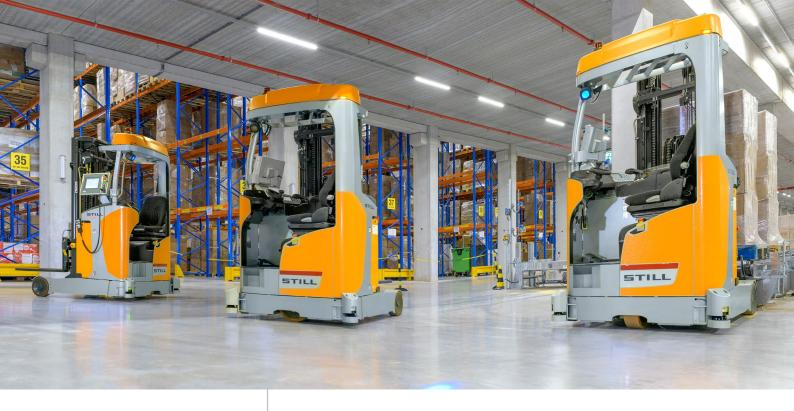
A total of twelve warehouse trucks are used; 7 STILL FM-X reach trucks, for the supply of pallets to the bulk warehouse, and 5 MX-X narrow aisle trucks for fully automatic loading and unloading in the bulk warehouse with 32 passageways.
