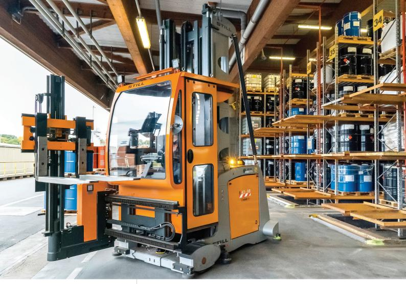
The stainless steel coated prongs prevent sparks from being generated by shock and friction contact.
