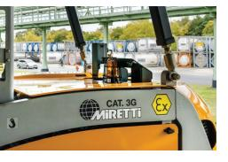
The potential ignition sources in the MX-X must be shielded and encapsulated against the explosive gas mixtures for category 2 hazard areas based on explosion-proof equipment category 3G.
