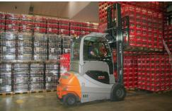
Other features include touch control, an electromechanical parking brake, exclusive seat version, LED road lights, hydraulic fork cushioning, GPRS terminal power supply and hydraulic fork positioners. Five-ton lift trucks are also raised to give the driver better visibility and a clear view of operations.
