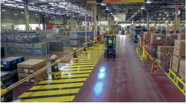
The forklift trucks are fitted with a STILL SafetyLight, a visual warning system which uses a bright spot on the ground to warn of approaching trucks.
