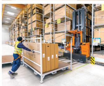
To pick the bicycles, the stake racks and the MX-X were specially designed by STILL.
