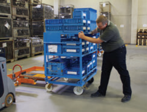
Up to 5 connected "E-type frames" can each accommodate one large or two small order picker trolleys.
