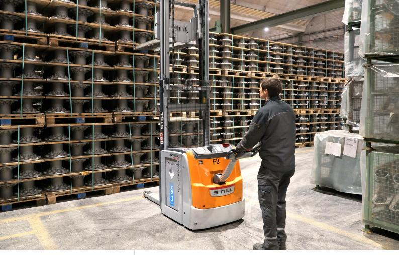
The maintenance-free Li-Ion batteries of the 23 new EXV 20 warehouse trucks can be charged to 50 percent of their capacity in just 30 minutes.
