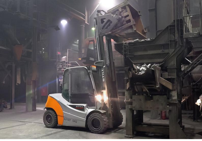
The RX 70 tilting device hydraulics are also protected from flying sparks and falling casting residues.
