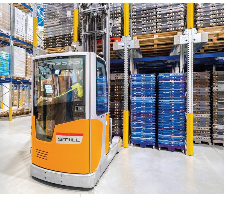
All pallets can be handled either lengthwise or crosswise thanks to the trucks' adjustable prongs.
