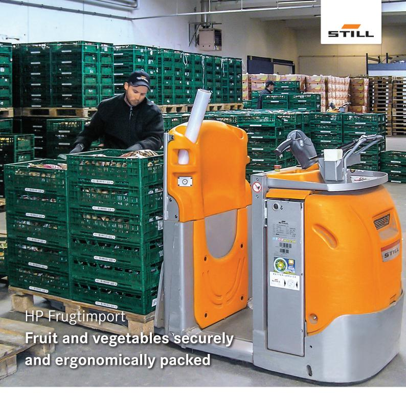
The COP-H 10 low level order picker has a low access point on either side, and good storage options for order slips, film and adhesive tape.
