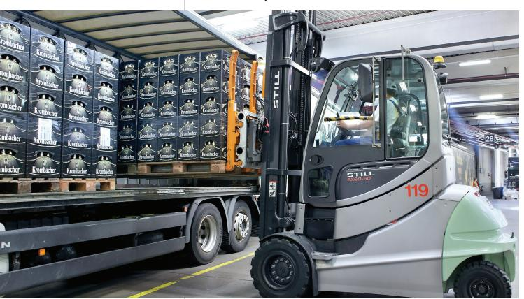
The specially reinforced lifting equipment contributes to an increase in nominal load capacity, amongst other factors. It can lift up to 1150 kg more depending on the lifting height.
