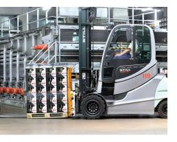
The RX 60-50/600 is a compact electric counterbalanced forklift truck with an extended load centre of 600 mm and a load capacity of up to five tonnes.
