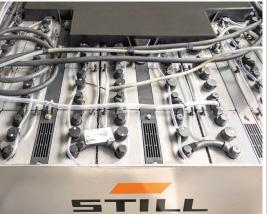
The air cooling system of the STILL Power-PlusLife battery reduces the core temperature by up to 20°C.
