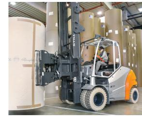
The highly manoeuvrable RX 60-80 supplies the production machine with paper rolls.
