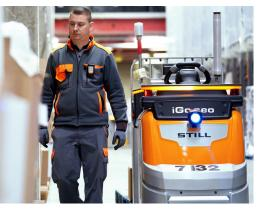
The intuitive remote control can be used to set the truck's ideal position for picking orders, i.e. at the start, middle or end of the pallets on the truck.
