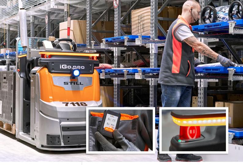
The hybrid tracking system also features significantly improved operator recognition: the combination of the motion tracking sensors on the vehicle and the radio signals from the remote control tracks employee positions one-on-one – even during heavy traffic.
