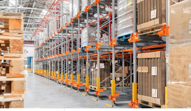
Safety standards, consolidation and flexibility have all significantly improved through the use of the STILL Pallet Shuttle channel storage system in comparison to manually operated drive-in racks.
