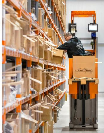
In the wide-aisle warehouse, order picking is carried out with the EK-X, while the FM-X takes care of stock replenishment.
