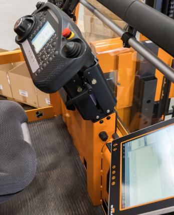
The ALS and AFC assistance systems in use with the MX-X Very Narrow Aisle Truck significantly increase the handling capacity.
