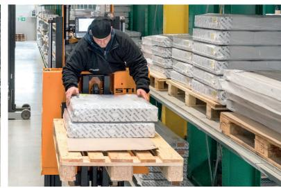
In the lower rows of racking, the EK-X carries out order picking of heating elements. At the same time, the FM-X coordinates replenishment of stock in the upper rows of racking. The 1.27 metre-wide FM-X and the 1 metre-wide EK-X can both manoeuvre around the 3.68 metre-wide aisle at once.
