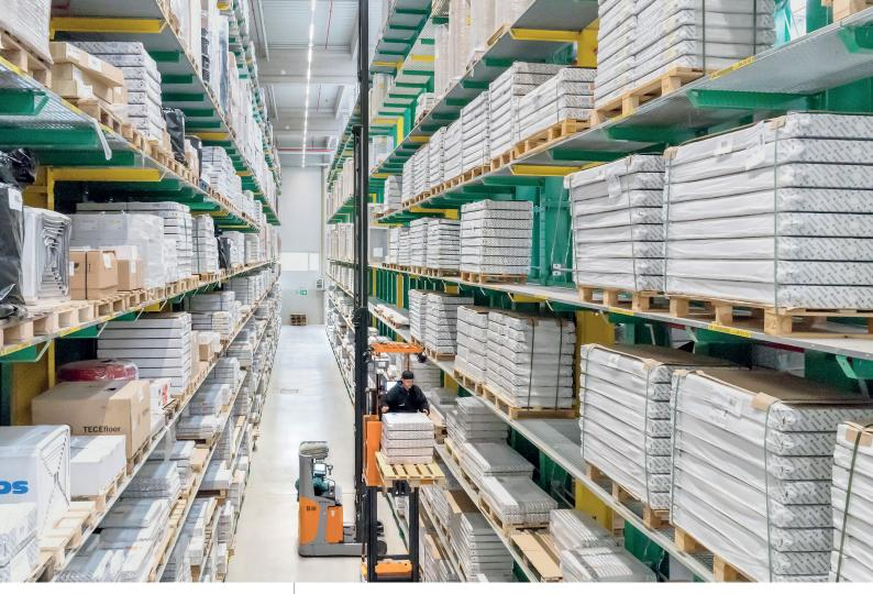
With its lateral fork camera, the FM-X 20 reach truck can store heavy pallets weighing up to 400 k at heights of up to 13 metres.
