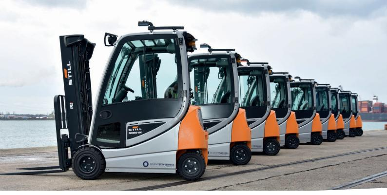
The new combination axle on the RX 20, ensures the smallest turning radius in its class, providing Solent with phenomenal manoeuvrability.
