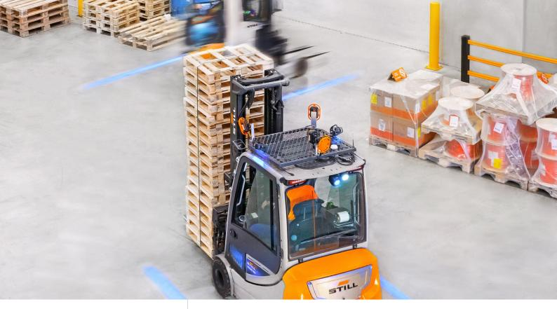
The trucks were equipped with a radio-based assistance system for collision protection. In addition, the warning zone light provides a warning of approaching trucks.
