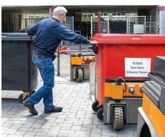
↑ Easy to secure loads: if the bracket hasn't been lowered, the tow tractor is not able to start.
