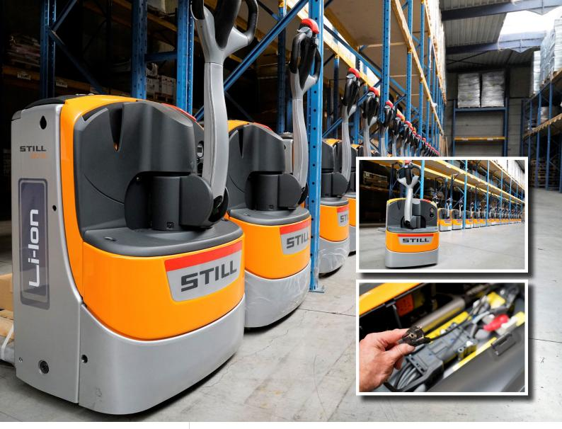
Thanks to a built-in charger, we are able to charge the trucks whenever necessary at any 230-volt power socket.
