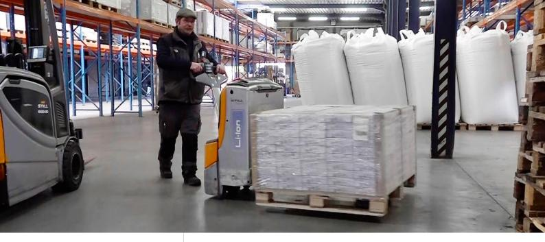
Compared to conventional batteries, the investment costs are around 30 percent higher. However, V1000 has found that this factor is offset by the benefit of short charging times of around half an hour.
