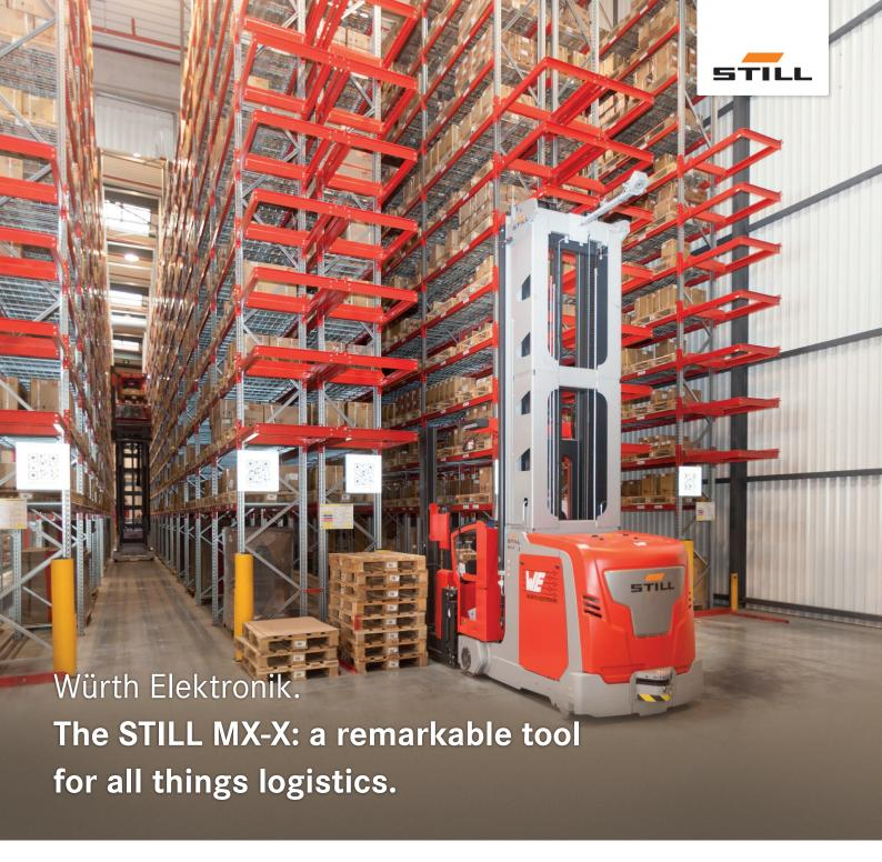
The very narrow aisle truck for high shelving is designed to facilitate warehouse management for industrial companies.
