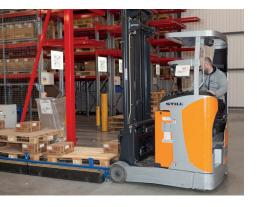
Incoming and outgoing goods were separated. The STILL FM-X 10 reach truck picks pallets off the conveyor belt at the dispatch area and loads them onto the console at the end of the palletiser.
