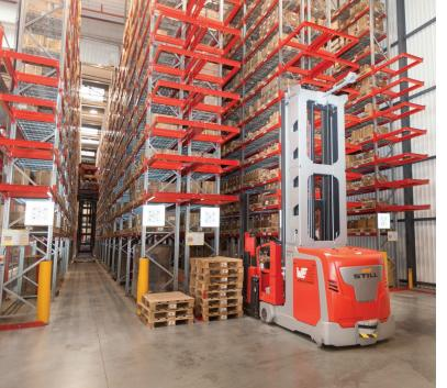
Both STILL MX-X VNA-trucks are provided with a motor-operated rear-view camera: the faster the truck goes the wider the camera's angle of vision becomes.
