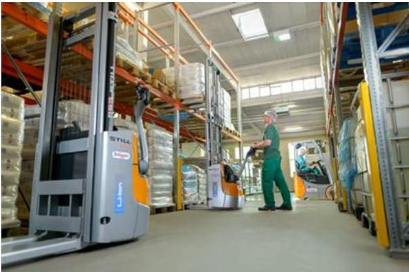
Picture 2: Thirty-nine different Li-Ion truck models with different lift heights, fork lengths and battery capacities are currently in use.
