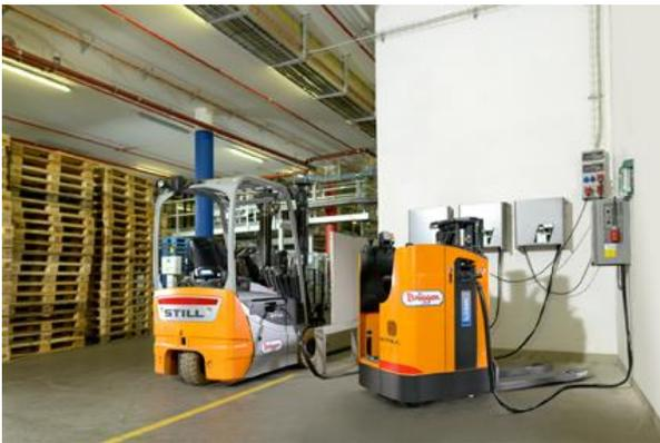
Picture 4: In contrast to lead-acid batteries, intermediate recharges are possible in any state of charge. All that needs doing to charge them is to connect them conveniently via the externally accessible charging connection.
