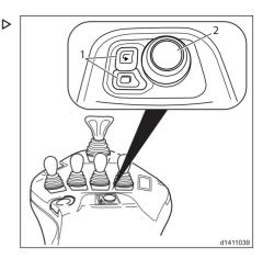
The drive controller is operated using the rota- ▷ ry/push button (2), the "Back" button (1) and the "Switch" button (3).
