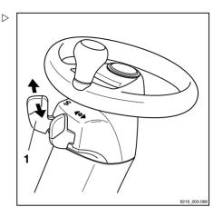
The turn indicators and the turn indicator display (2) or (3) on the display-operating unit flash.
