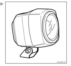
Depending on the configuration of the truck, the STILL Safety-Light 4Plus® automatically switches itself on when the truck is moving. This means that, during reverse travel (variant), for example, it can be used as an additional light for the working spotlight for reverse travel. The STILL Safety-Light® or the STILL Safety-Light 4Plus® can also be switched on and off on the display-operating unit.
