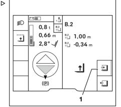
Select the desired area of the warehouse either in the function menu "Load ► easy Target" or via the favourites. The adjacent example shows the selection via a favourite (2).
