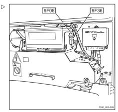
Sheathed-element heater plug (only on diesel trucks), 25 A
