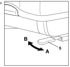
A Longitudinal horizontal suspension activated B Longitudinal horizontal suspension blocked
