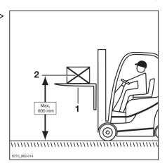
Reversible fork arms (1) can be used to reach an additional lift height. The reversible fork arms are installed on the fork carriage in the same manner as standard fork arms. Loads may be lifted on and beneath the reversible fork arms. The mast is lifted and tilted in the same manner.
