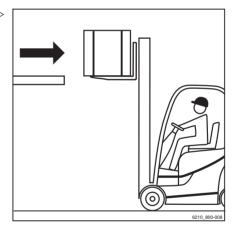
Lower the load while maintaining ground clearance.
