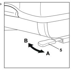
Longitudinal horizontal suspension activated Longitudinal horizontal suspension blocked
