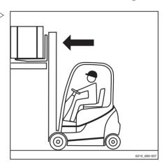
Lift the fork carriage until the load is resting entirely on the forks.
