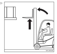
Insert the fork as far under the load as possible. Stop the truck as soon as the fork back is resting on the load. The centre of gravity of the load must be positioned between the fork arms in the middle.
