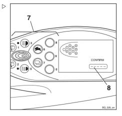
If the driver PIN entered in the CONFIRM submenu does not match the driver PIN entered previously in the NEW CODE submenu, the message INVALID will appear.
