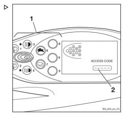
If an incorrect driver PIN is entered, the message INVALID appears for a short time. When the message goes out, the driver PIN can be re-entered.
