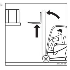
Insert the fork as far under the load as possible. Stop the truck as soon as the fork back is resting on the load. The centre of gravity of the load must be positioned between the fork arms in the middle.
