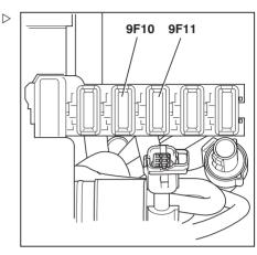
9F10 Air conditioning (variant), compressor / condenser, 20 A
