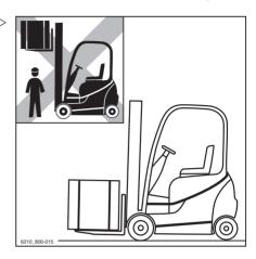
Lower the load until it rests securely on the rack.
