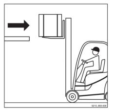
Lower the load while maintaining ground clearance.
