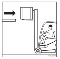
Lower the load while maintaining ground clearance.
