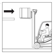
Lower the load while maintaining ground clearance.
