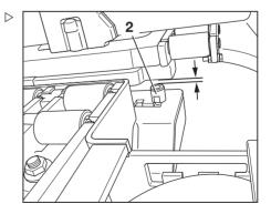
The external roller channel is placed correctly. ▷
