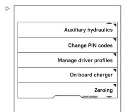
Press the softkey for the assistance function for which the zeroing is to be performed, e.g. Load weight.
