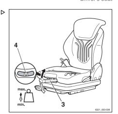
The seat automatically adjusts to the driver's weight.
