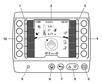
The display-operating unit is operated using the control and enter keys (5...8) and the soft-keys (4, 10). The display (2) shows information about the current driving programme, load programme and the configuration of the favourites bars (1, 3). The brightness sensor (9) automatically adjusts the brightness of the display based on the truck's surroundings.
