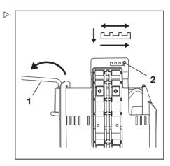
Place the battery changing bridge so that the indexing bolt (2) is in the corner of the edge.
