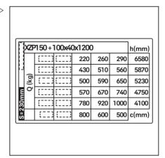
Residual load capacity rating plate for large sideshift, S = 230 mm
