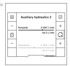
The return flow is displayed in addition to the supply flow at full brightness.
