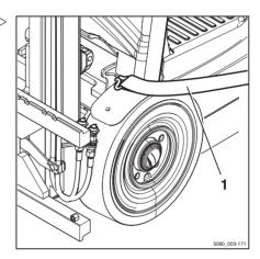
Loop lashing straps (2) around the rear of the truck within the chassis contour and lash the truck to the front.
