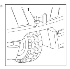
Access to the battery compartment and battery male connector
