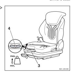
The seat automatically adjusts to the driver's weight.
