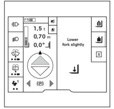
If the calculation was successful, the measured weight of the load (1) is displayed.
