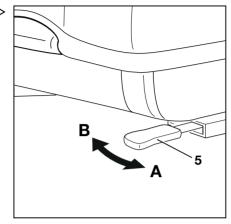
Longitudinal horizontal suspension activated Longitudinal horizontal suspension blocked
