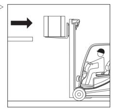
Lower the load while maintaining ground clearance.
