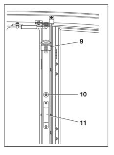
Push in the latch. Push the front door section (6) outwards and swivel it 180°.
