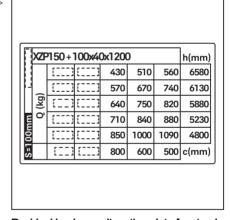
Residual load capacity rating plate for standard sideshift, S = 100 mm
