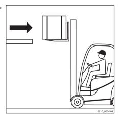
Lower the load while maintaining ground clearance.
