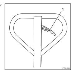
Pull operating lever (1) upwards. The initial lift must retract again without jerking.
