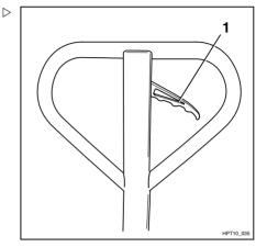
Pull operating lever (1) upwards. The initial [ lift must retract again without jerking.
