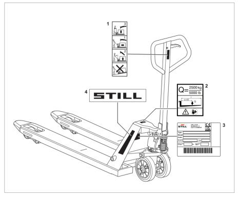
Decal information: Lower load/Transport load/Lift load/Do not drive on slopes
