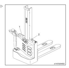
Turn the key switch (1) to the ON position; the battery indicator light will come on.
