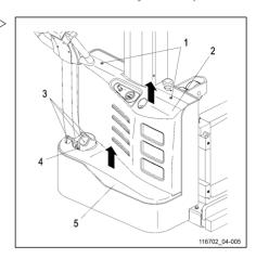
The emergency lowering screw is located on the solenoid valve(2).
