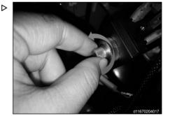
Unscrew the two large flat-head screws(1) and pull out the cover(2).
