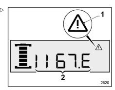
Specific alarm relating to charging via the on-board battery charger (if present). The alarm indicator light (1) lights up on the display. Field (2) displays Error and the segments (3 and 4) flash. The alarm indicates that the truck has problems with charging via the on-board charger. Switch the truck off and on again. If the alarm appears again at start up, contact the technical service centre.
