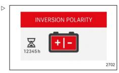
Polarity reversed with charger disconnected.
