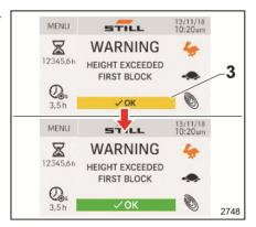
The symbol (3) indicates that the second lift cut-out has been exceeded.
