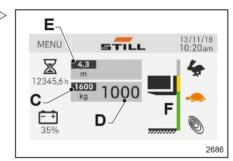
Third example: The load on the forks (D) of 1400 kg may be raised to a maximum of 3.1 m (E). The zone (F) indicates that the 1400 kg load may be raised to the green zone, which can be easily identified on the coloured adhesive string (G).
