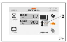
The warning indicates that the fork lift height setting for the second cut-out has been reached. In order to raise the forks higher, press and hold the yellow bar (3) with "OK" until it turns green. When it is released, the display returns to the main screen.
