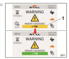
The warning with the symbol (1) is displayed until the forks are lowered below the preset cut-out height.
