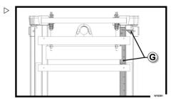
First example: The load on the forks (D) of 500 kg may be raised to a maximum of 5.4 m (E). The zone (F) indicates that the 500 kg load may be raised up to the red zone, which can be easily identified on the coloured adhesive string (G).
