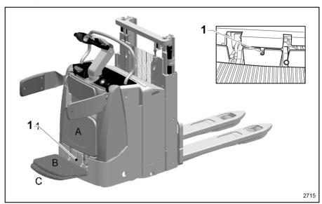
The platform can take three positions, **A**, **B** and **C**:
