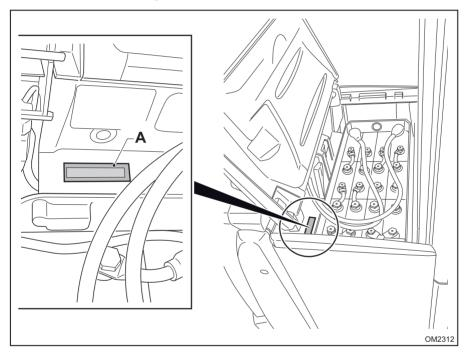
The truck's serial number is marked (A) on the chassis frame.
