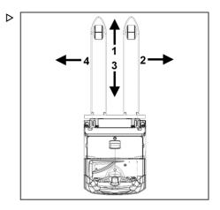
Definition of directions for EXV-SF, EX- Vi-SF and EXV-SF D versions with platform lowered and when the operator is on board the truck
