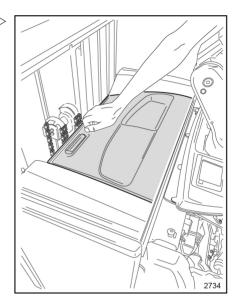
If you need to recharge the battery, disconnect the battery plug and socket by means of the appropriate handle.
