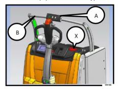
The specific commands for the additional hydraulic equipment are positioned on the keypad (A) fixed on the accessories mounting bar (B). In case of emergency, press the relevant button (X)
