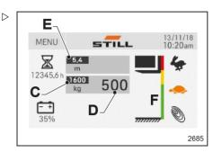
Second example: The load on the forks (D) of 1000 kg may be raised to a maximum of 4.3 m (E). The zone (F) indicates that the 1000 kg load may be raised up to the yellow zone, which can be easily identified on the coloured adhesive string (G).
