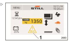
The red flashing warning triangle (1) on the display indicates that the load on the forks has reached or exceeded the limit of the maximum capacity of the truck.
