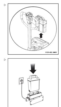
Plug into charging stand and charge (110/220V 50/60HZ).
