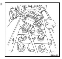
Operate and pull the locking handle (2) in the direction indicated by the arrow.
