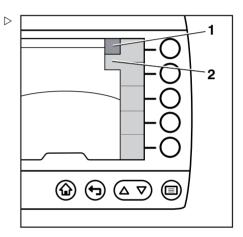
The display-operating unit can display a maximum of five menu items simultaneously. If there are more menu items within a menu, the scroll indicator (1,2) appears. This indicator appears only if there are additional menu items. Use push buttons  $\triangle$  and  $\nabla$  (3) to scroll.
