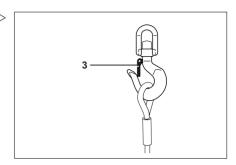
Adjust the length of the harnesses so that the bridge piece is vertically above the centre of gravity of the industrial truck. This will ensure that the industrial truck remains level when it is being lifted.
