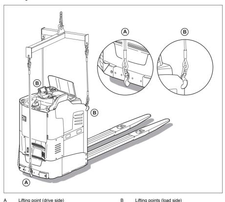
Α Lifting point (drive side) Lifting points (load side)
