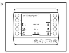
To reset a value, press the "Clear" Softkey. ▷ The value is set to "zero".
