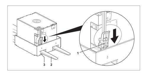
Insert the battery male connector of the battery into the dummy plug (1) on the battery plate.
