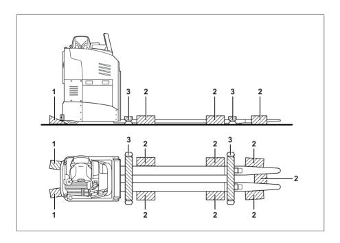
For transportation by lorry or goods wagon, the industrial truck must be secured with wedges and tension belts.
