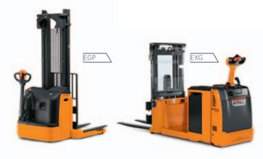
The EXG – a pedestrian pallet truck with extra possibilities. The EXG is a powerful piece of equipment which offers all the advantages of a traditional counterbalanced forklift combined with a manually operated warehouse organiser. High residual load capacity and the option of using commercially available accessories are just two of its individual strengths.
